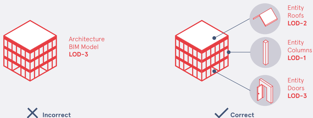
Figure 5. Simultaneity of different LOD of the entities in a BIM model
