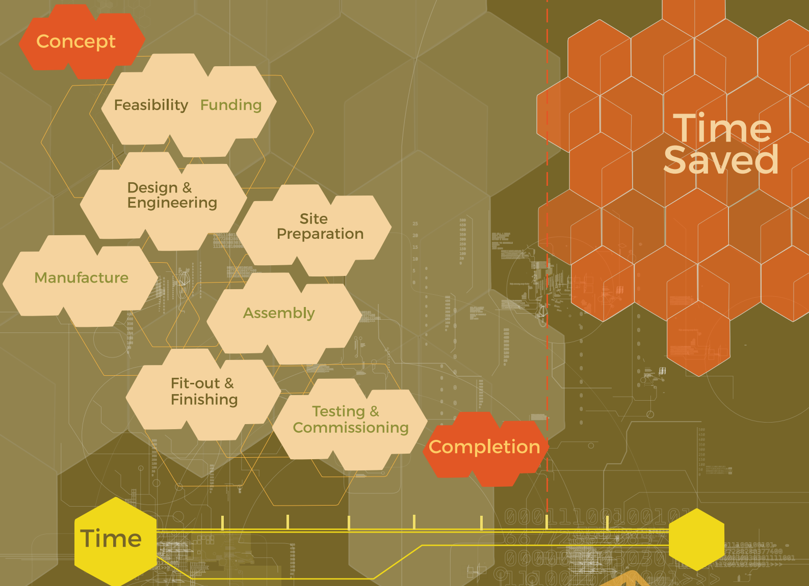
Figure R2 — Typical reduction in construction programme using DfMA
