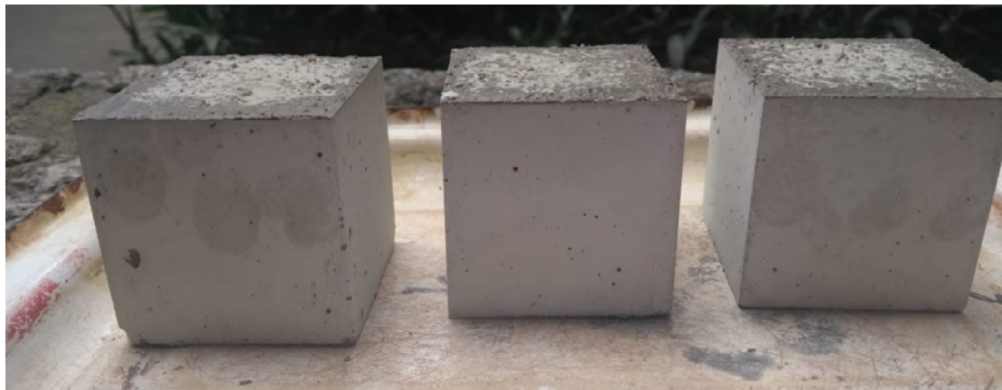
Figure 34: Best condition mortar (CFm30) to develop concrete
