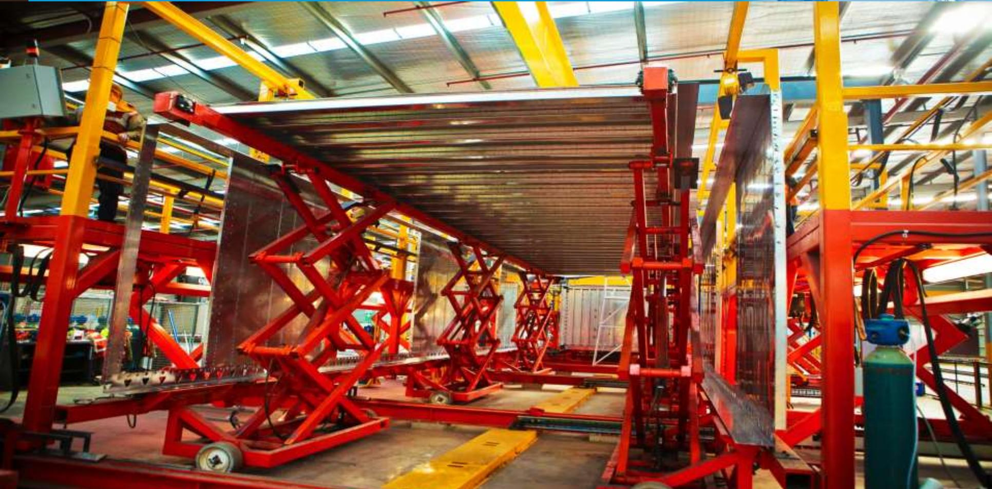
Panels held in position and welded into a unit
