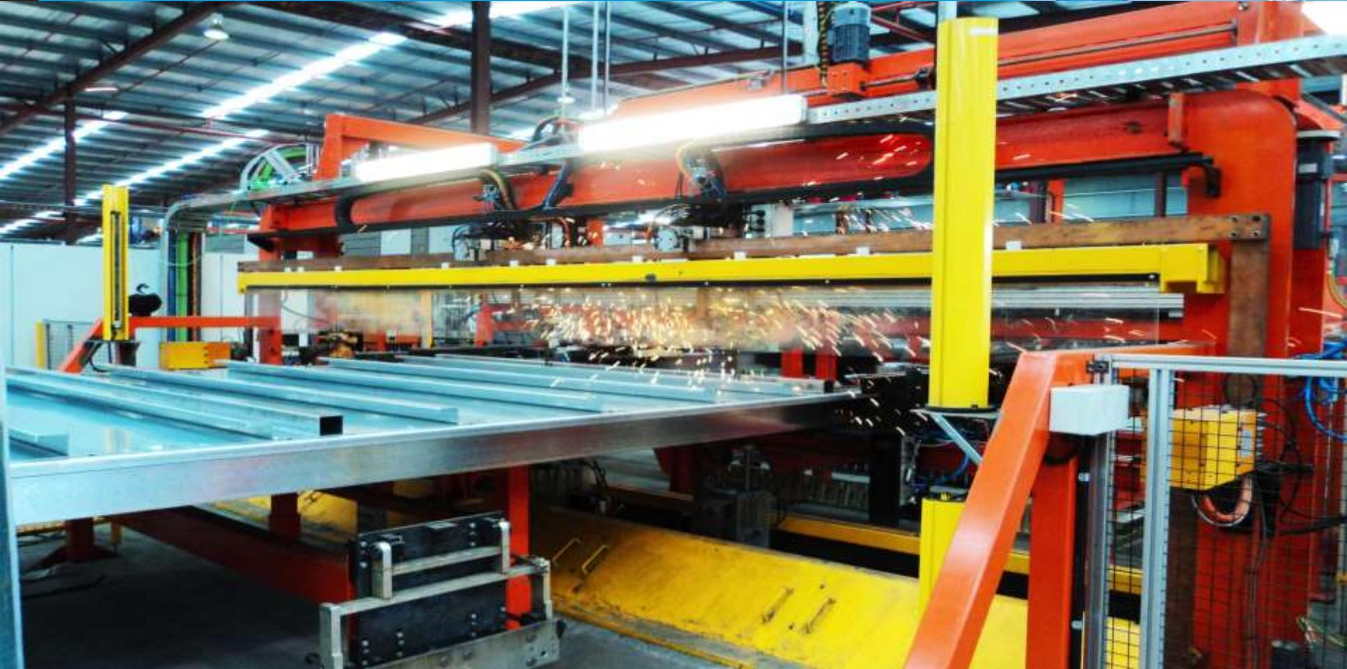
Completed panels placed into jig
