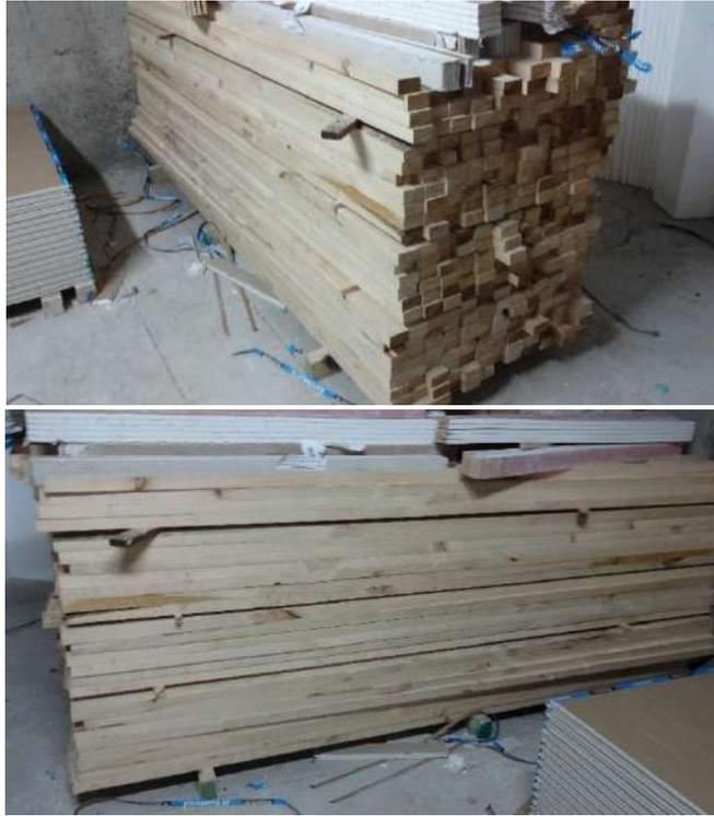
**Figura 17:** PINO CEPILLADO SECO 37 X 55 X 2.40 MT. (MCB0101) (CITEC-UBB)
