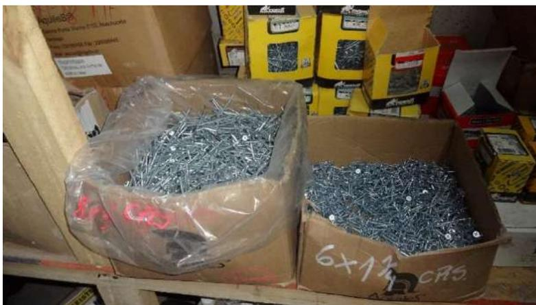
**Figura 22:** MDE0308 TORNILLO AUTOCORROSCANTE 6 X 1 1/4" H/FINO (CITEC-UBB)
